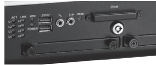
Swappable and Lockable SATA3 HDD/SSD, Audio jack, USB 3.0 and CFast
