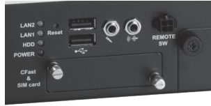
Removable CFast™, SIM slot and suspension 2.5" SATA HDD/SSD
